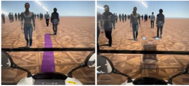
Figure 1. Types of visual information to reduce the anxiety of PMV passengers. The left shows the “Path” type describing the future position as a line on the ground, and the right shows the “Follow” type describing the future posture angle and its position as a leading PMV.
