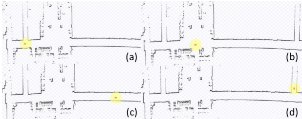
Fig. 4. Fuzzy neural network follower controller training in ROS Stage using the automobile factory corridor map.
